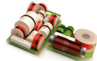
The cross over is paramount to the sound quality. It uses the finest components and is tuned using real time digital filtering techniques, MLS measurements and critical listening.
